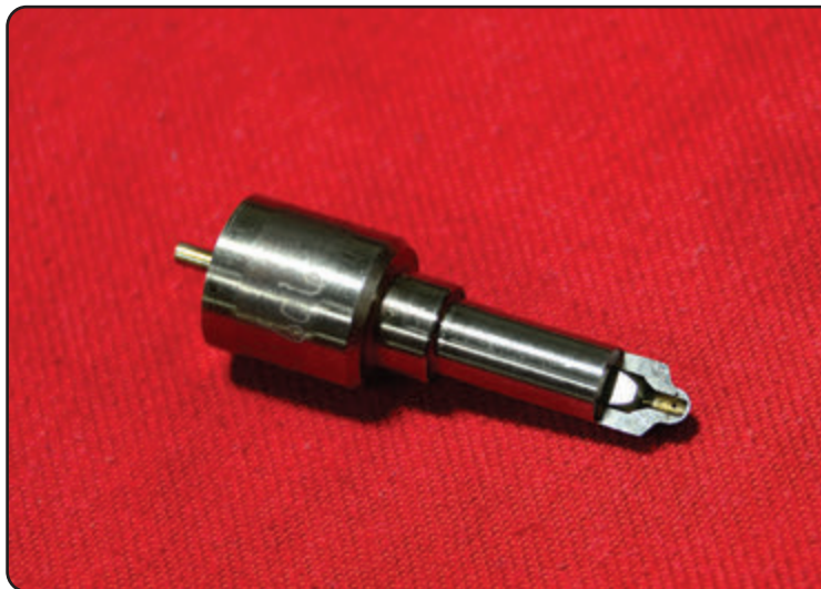
16 This injector has a sac tip, which is generally more durable than the sacless type. A sac tip doesn't have a tunnel or trough for the fuel, but instead a cone-shaped area for seating the pintle.
