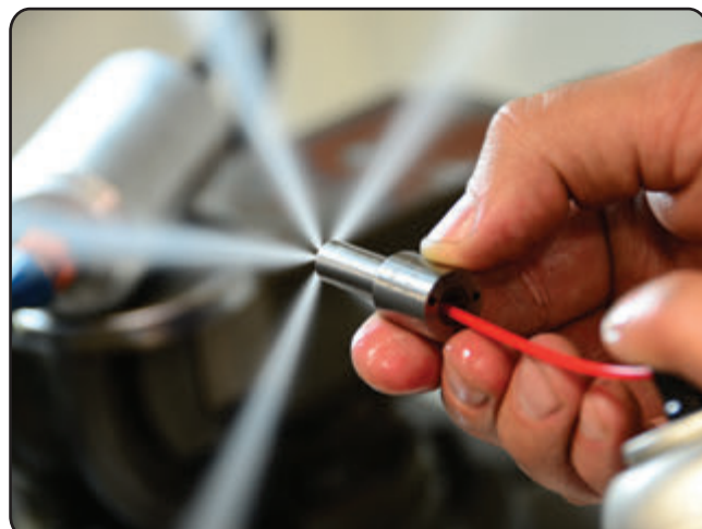
12 A factory injector might have only three holes in the nozzle, while a performance unit anywhere from four to 12 holes.
