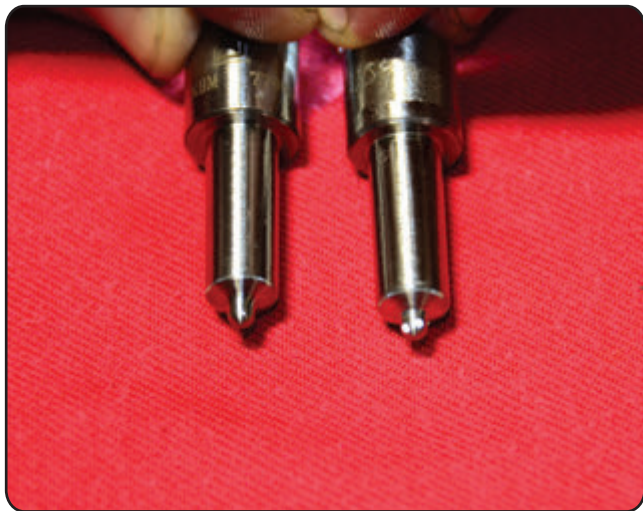
13 By shining a flashlight through each injector body, you can see larger points of light on the tip at right, showing the difference in volume. Fuel flow can be increased by anywhere from 20 to 500 percent, depending on the application.
