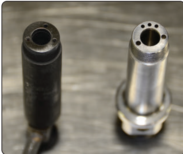
1 At left is a stock, IH injector body with a single feed. At right, additional fuel-feed holes are evident in a Scheid billet tri-feed injector body.
