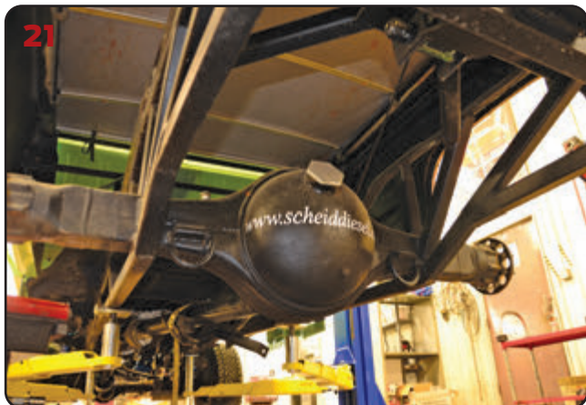
20 & 21 Scheid Diesel handles about 30 or more sled-pull trucks. The Super Ram shown here, owned by Rod Tarr, runs in the 3.0-inch Inducer class, and grabbed third place in ITPA points. To handle as much as 2,750 horses, Scheid adds substantial bracing around the Profab SQHD rearend.
