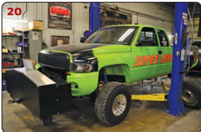
20 & 21 Scheid Diesel handles about 30 or more sled-pull trucks. The Super Ram shown here, owned by Rod Tarr, runs in the 3.0-inch Inducer class, and grabbed third place in ITPA points. To handle as much as 2,750 horses, Scheid adds substantial bracing around the Profab SQHD rearend.
