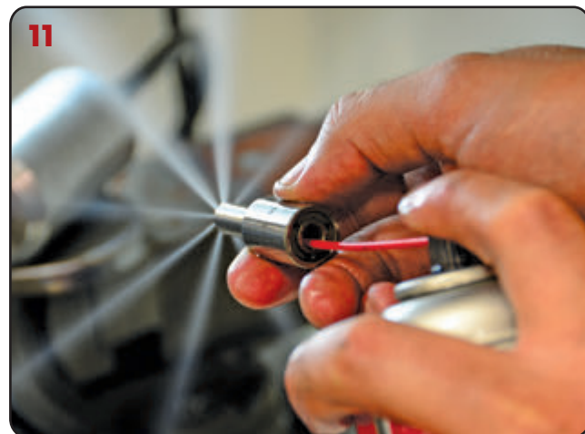
10 & 11 Using an aerosol can of cleaning fluid to illustrate, you can see the difference in the volume of spray. At left, the jets have a fairly uniform size, but at right, the top two jets are slightly wider, since the orifices have been enlarged to deliver more fuel.
