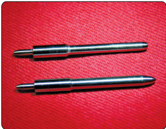
14 These pen-shaped units, called pintles, act like valves that lift up from the seat in the injector tip to allow a precise pulse of fuel to flow through the nozzle tip.
