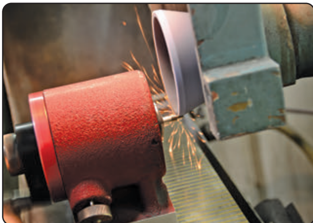
18 Removing material from the pintle tip increases lift, resulting in a bigger pulse width.
