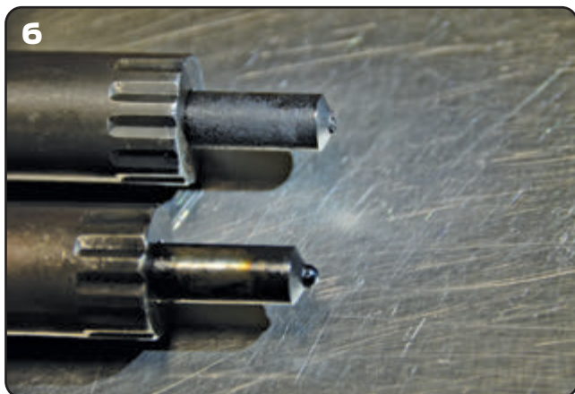
5 & 6 Look closely at the tips; note how one of them has burst. These are the "sac type," referring to the area where the pintle or pin seats within the injector. This type is considered to be more durable than the "sacless" VCO (valve closes orifice) nozzle.
