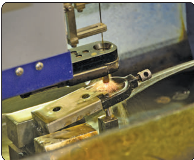
17 With the nozzle orifices enlarged, the feed passage in the injector body might become a bottleneck for fuel flow, so Scheid adds up to two extra feed passages with the EDM.
