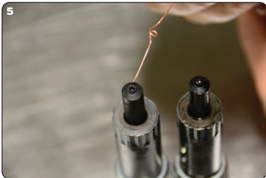
5 & 6 Look closely at the tips; note how one of them has burst. These are the "sac type," referring to the area where the pintle or pin seats within the injector. This type is considered to be more durable than the "sacless" VCO (valve closes orifice) nozzle.
