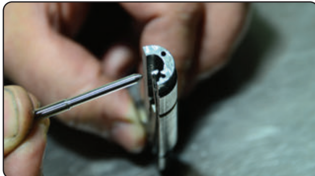
3 Here's another view of a damaged injector, caused by an incorrect spray orifice and/or a quick-rate pump cam. Static pressure on an injector starts at 4,500 psi, but during operation can go as high as 15,000 psi, putting considerable load on the assembly.
