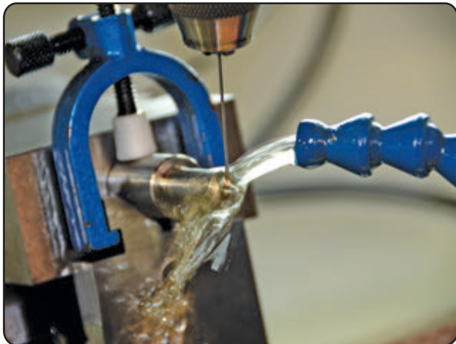
7 Electrical Discharge Machining is a very precise way to enlarge or add holes in an injector tip, and also change the spray pattern. Careful inspection with a 25X power magnifying glass helps to evaluate modifications made to the injector nozzle.
