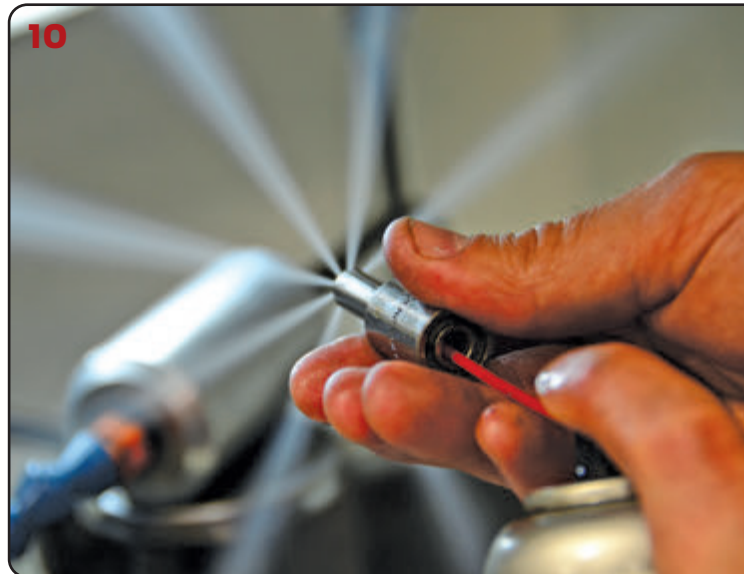
10 & 11 Using an aerosol can of cleaning fluid to illustrate, you can see the difference in the volume of spray. At left, the jets have a fairly uniform size, but at right, the top two jets are slightly wider, since the orifices have been enlarged to deliver more fuel.
