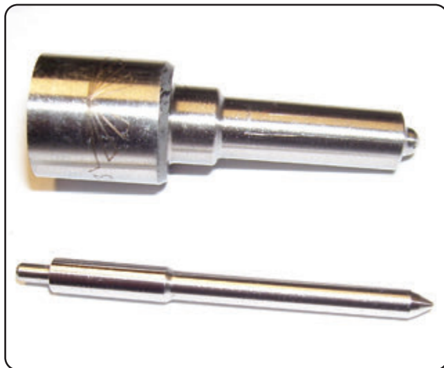
22 This tip for a 12V Cummins uses a five-hole, sac-type nozzle that has proven to be one of the best all-around nozzles, Scheid says. It has supported 50-hp gains, and also dyno runs up to 800 hp when combined with twin turbos and other performance parts.
